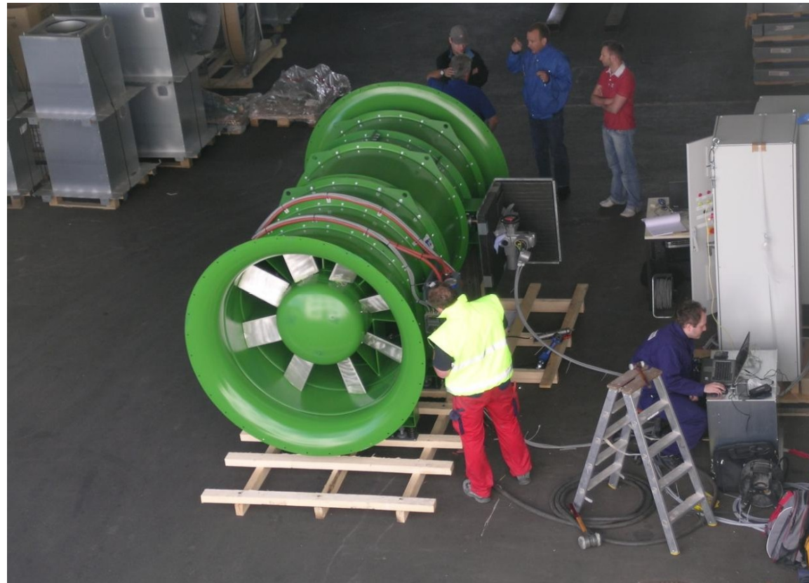
Picture of metro fan testing
